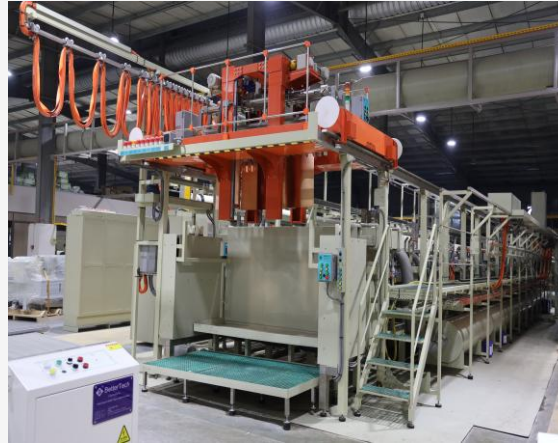
Copper Plating Line with Reverse Pulse Plating
